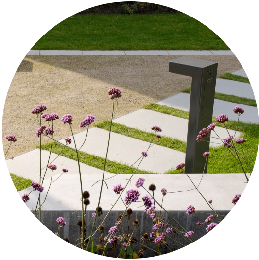
Bollard Lighting: the walkway down to the common viewing pavilion is lit with bollards running down one side of the path
